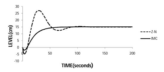
Fig: 3 Comparison between Z-N and IMC method
